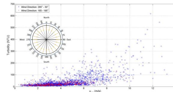
Figure 5: Turbidity versus wind velocity  $u_{10}$ , separated based on wind direction, in Terrebonne bay for measurement from 24/8/2010 to 31/12/2010. Northerly wind (wind direction  $\sim 285^\circ - 30^\circ$ ) associated with large turbidity values, while southerly wind (wind direction  $\sim 165^\circ - 195^\circ$ ) only causes mild changes in turbidity.
