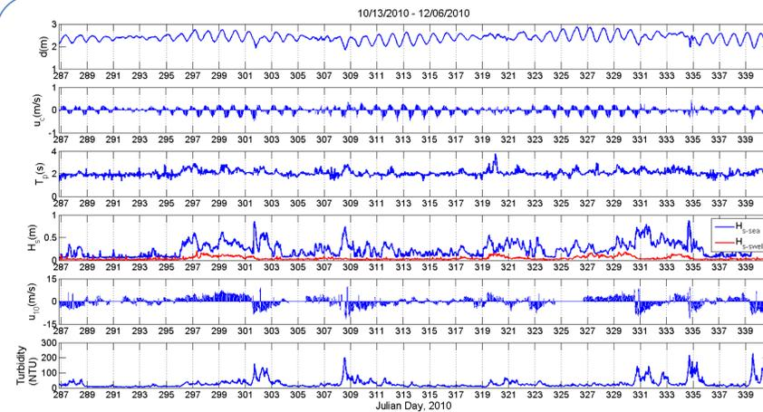
Figure 3: Time series of measurement from 13/10/2010 to 6/12/2010. From top to bottom: 1) Water depth  $d$ , 2) Current velocity/direction  $u_c$  at 1.09 m from bed, 3) Wave peak period  $T_p$ , 4) Significant wave height  $H_s$  for sea and swell, 5) Wind velocity/direction  $u_{10}$ , and 6) Water turbidity. Wind and current vectors show both magnitude and direction.
