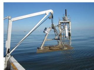
Figure 2: Sontek Triton ADV installed on tripod stand.
