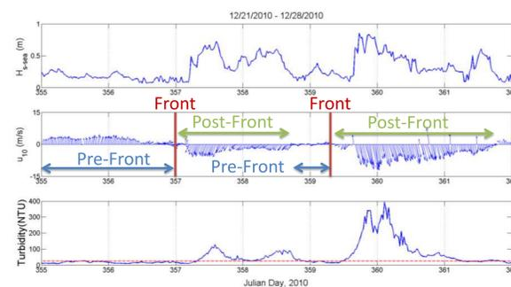
Figure 6: Two cold front passage in Terrebonne bay from 21/12/2010 to 28/12/2010. Fronts (red vertical lines) and their pre and post front phases are illustrated. From top to bottom: 1) Sea significant wave height  $H_{s-sea}$ , 2) Wind velocity/direction  $u_{10}$ , and 3) Turbidity. Increases in wave height and turbidity can be seen in post-front phase. Horizontal dashed line in plot (3) represents average turbidity for wind direction between  $135^\circ$  and  $225^\circ$  equal to 23.7 NTU.
