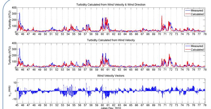
Figure 8: Comparison of predicted turbidity with measured turbidity in Terrebonne bay from 14/2/2010 to 19/3/2010. From top to bottom, 1) predicted turbidity using wind velocity  $u_{10}$  and wind direction, 2) predicted turbidity using only wind velocity, and 3) wind velocity vectors. Except for first peak, both method predict all turbidity peaks with good accuracy.
